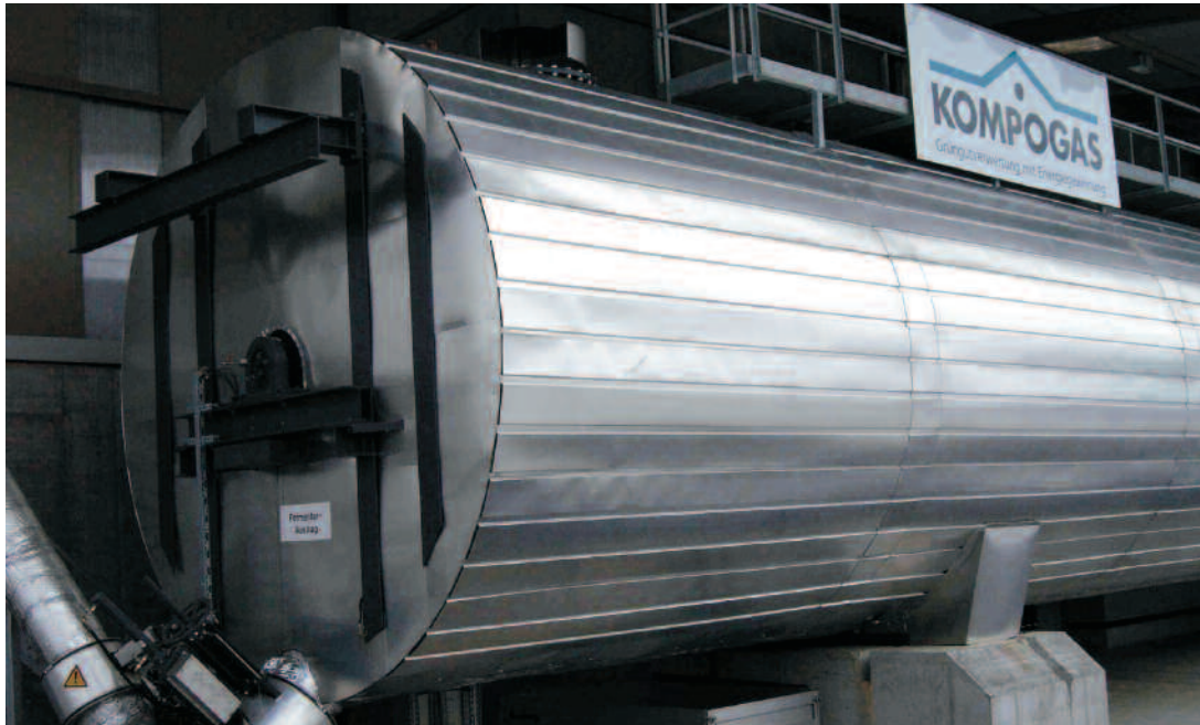
Fig 4 Anaerobic digester suitable for treating five tonnes/year of biowaste (including food)
